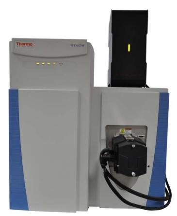
**Fig. 1** MA3100 IMS analyzer and control electronics shown interfaced with a Q Exactive<sup>TM</sup> orbitrap MS. Ion mobility devices from Excellims are now available for a range of Thermo Scientific<sup>TM</sup> trapbased instruments.
