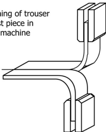
FIG. 2 Trouser Tear Test Specimen
