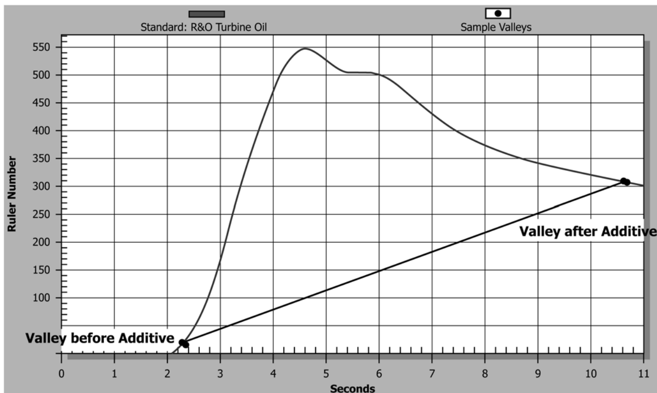
FIG. 1 Hindered Phenol Voltammetric Response in Basic Test Solution with Blank Response Zeroed
