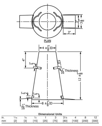
FIG. 1 Mold for Slump Test
